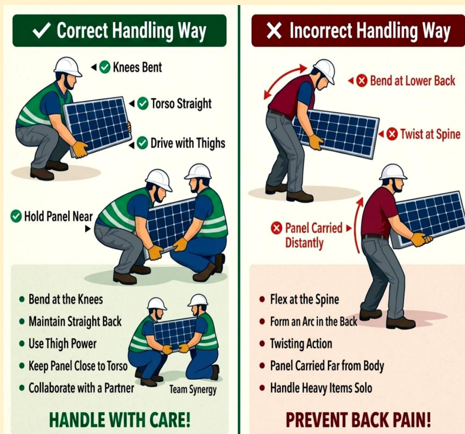
Figure 3.10: Safely lifting of Solar Panels
