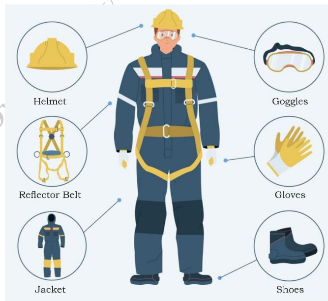
Figure 3.1: PPE Kit for Solar PV Installer (Civil)
